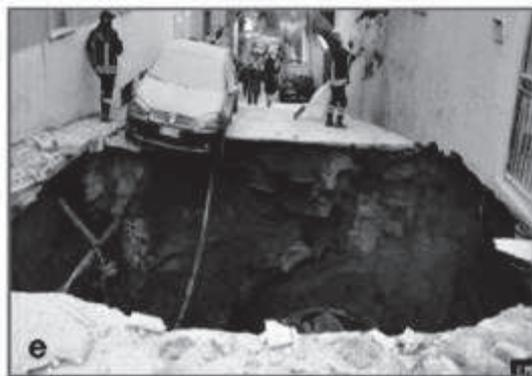
**Fig. 4.16.** Cave collapse in weathered Quaternary L'Aquila Breccia at Via Campo di Fossa (Martelli et al., 2011).
